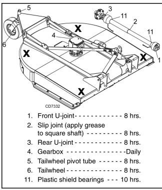
Figure 11. Jackstand Placement & Lubrication Points
